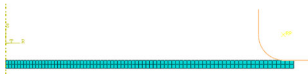
Fig. 15—Initial mesh of a blank used in gas-pressure bulge-forming simulation.
