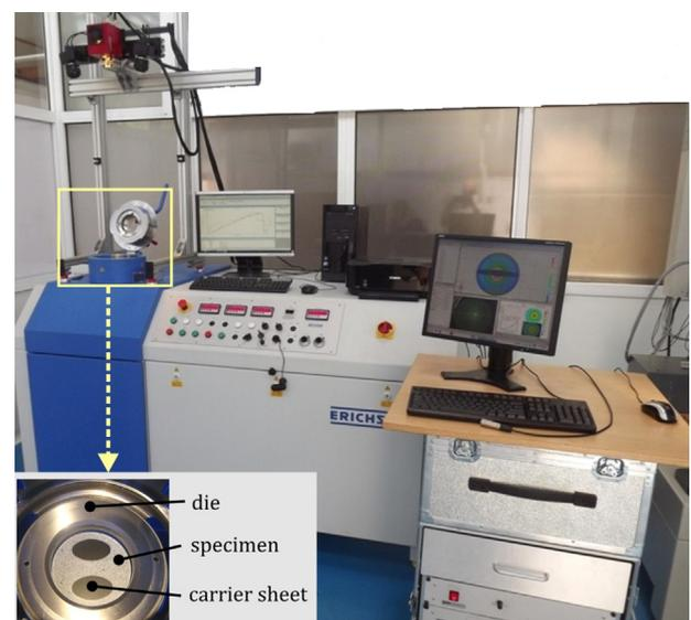
Fig. 7. Equipment used for the experimental determination of the FLCs.
