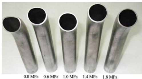
Fig. 6 Cross-section shapes of tubes bent under different pressures
