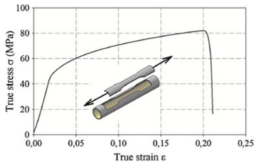
**Fig. 4** Stress–strain curve for an AA 1050 O aluminum tube
