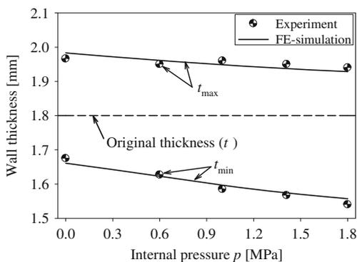
Fig. 9 Effect of the internal pressure on the wall thickness
