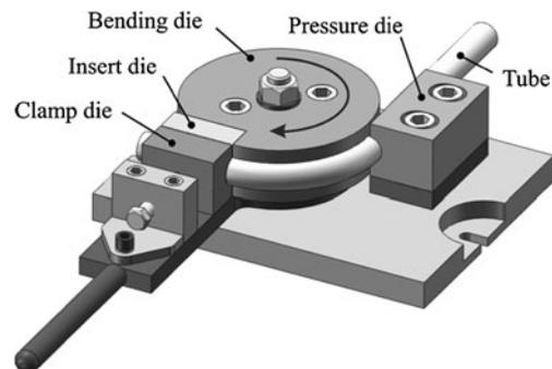
Fig. 1 Rotary draw tube bending device
