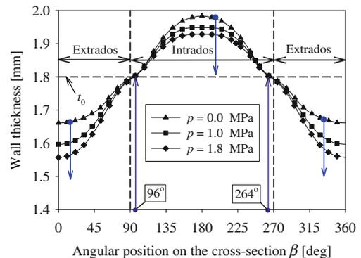
Fig. 11 Effect of the internal pressure on the change of the wall thickness at the level of the cross section located in the middle of bend region (see Fig. 3)
