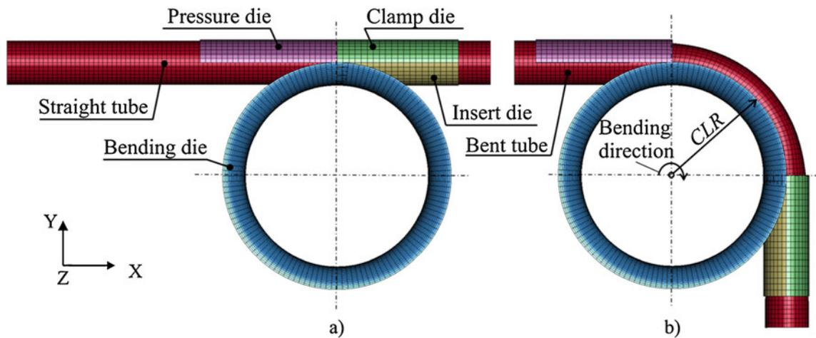
Fig. 5 3D FE model for the rotary draw bending of a tube: a initial position, b bending at 90°
