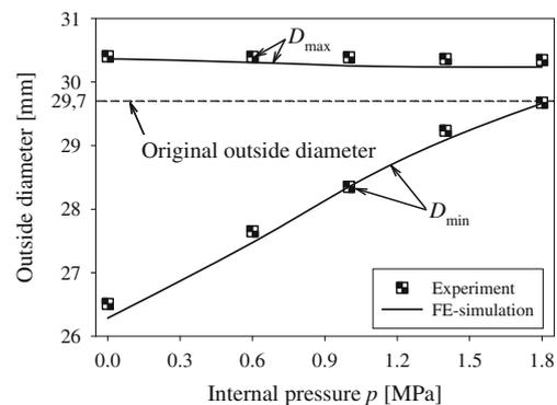
Fig. 7 Effect of the internal pressure on the cross-section deformation
