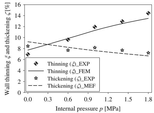
Fig. 10 Effect of the internal pressure on the wall thinning and thickening
