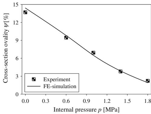
Fig. 8 Effect of the internal pressure on the cross-section ovality
