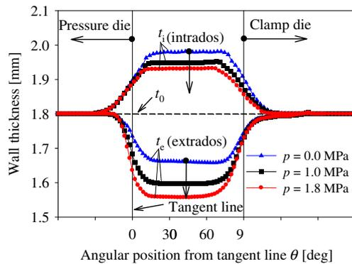
**Fig. 12** Effect of internal pressure on the wall thickness  $t_i$  and  $t_e$  at the level of the axial section shown in Fig. 3
